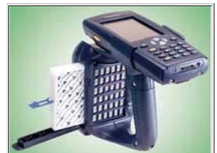
Commercial Launch: MTI Micro claims to be the first to market with a methanol cell that continuously charges a lithium-ion battery for an RFID reader. MTI's technology eliminates the pumps found in most DMFC cells and feeds methanol directly into the anode side of the cell.
