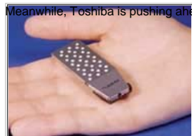
Tiny Package: Toshiba has developed an 8.5-gm DMFC for devices as small as digital audio players and headsets for mobile phones.
